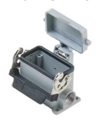
Surface mounting housing, C-TYPE series, with 1 lever, Pg29 x 2 cable entry, size "57.27", high construction, with metal cover
