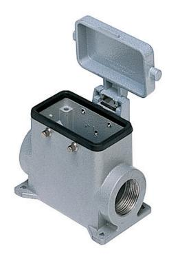
Surface mounting housing, C-TYPE series, with 4 pegs, Pg21 cable entry, size "57.27", high construction, with metal cover
