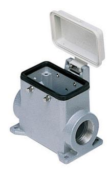
Surface mounting housing, C-TYPE series, with 4 pegs, Pg21  $\times$  2 cable entry, size "57.27", high construction, with plastic cover
