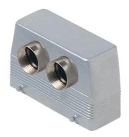
Hood, C-TYPE series, with 4 pegs, Pg21 x 2 double frontal cable entry, size "77.27", high construction
