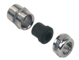
Complete cable gland, M20, for diameter 8-12 mm, 15 mm threading length
