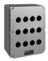
Box for control devices and signals, AC series, M32 cable entry, 12 holes for unit  $\emptyset$  22 mm, external dimensions 152x205x102 mm
