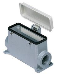
Surface mounting housing, 830V series, with 4 pegs, M32 cable entry, size "104.27", high construction, with plastic cover
